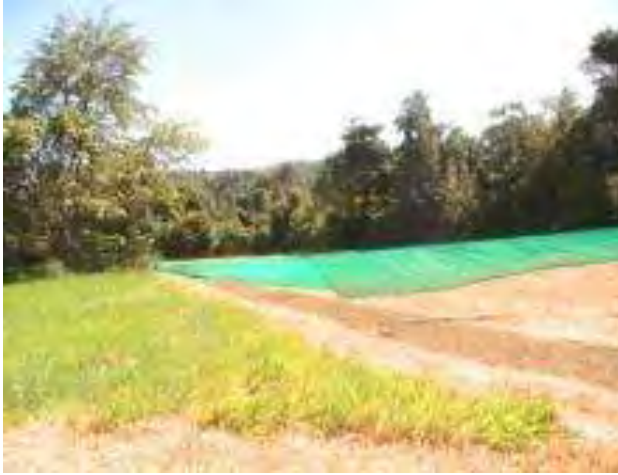
Figure 4.10 Fence sag test – no posts
