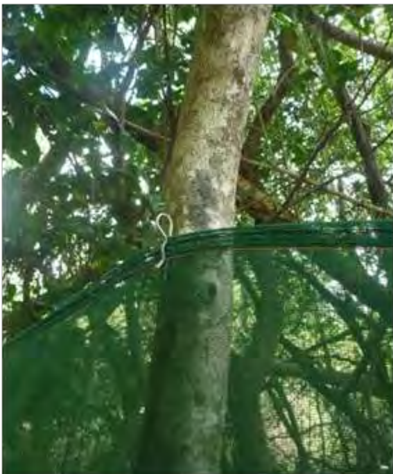
Figure 4.15 Shear clip attachment to tree using coach screw Untouched for 1½ years
