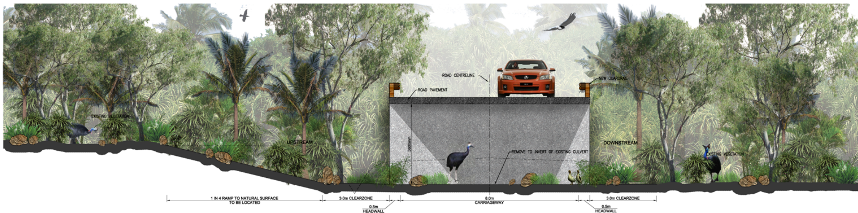
TYPICAL SECTION THROUGH UNDERPASS VERTICAL SCALE 1:20
