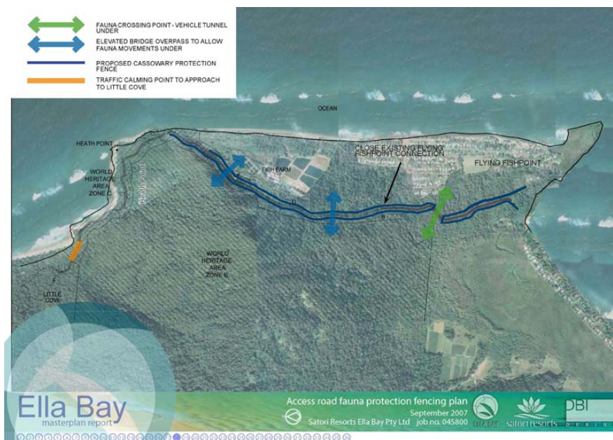
Figure 13. Elements of the Fence & Funnel Strategy. This involves fencing for most of the route and provision of fauna underpasses opposite the Flying Fish Point Reserve and south of Heath Point.
